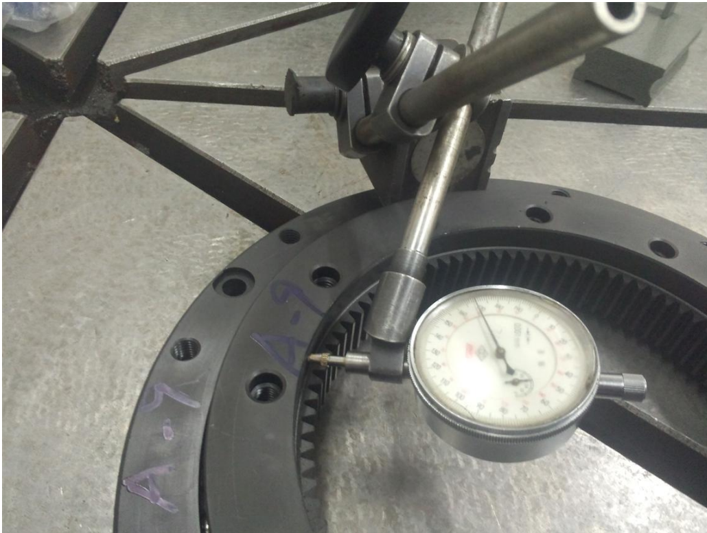
Test for the radial runout of inner ring
